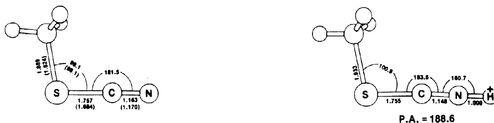
Fig. 1. 56 Calculated structures of neutral and protonated \text{CH}_3\text{SCN} and their proton affinities. Bond lengths are in Å and proton affinities in Kcal/mol. Experimental structural parameters of \text{CH}_3\text{SCN} 43 are shown in parentheses.
